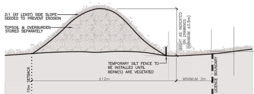
TYPICAL BERM SECTION N.T.S.
