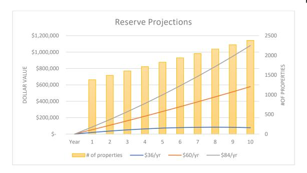
The storm sewer infrastructure in Thamesford and Embro is relatively new, ranging from 11 to 22 years, so the need to build a reserve for replacement is a long-ways away. In order to properly evaluate the system reserve required, a system evaluation (condition and cost) would be required. From the above table, it would appear that \$60 per year per property would start to build a reserve. If the operational costs get higher than estimated, the \$36 per year is not enough to cover costs.
