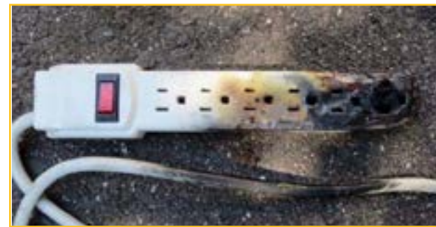
This extension cord caused a fire because it was connected to a space heater. Extension cords are not designed to take these heavy loads.
